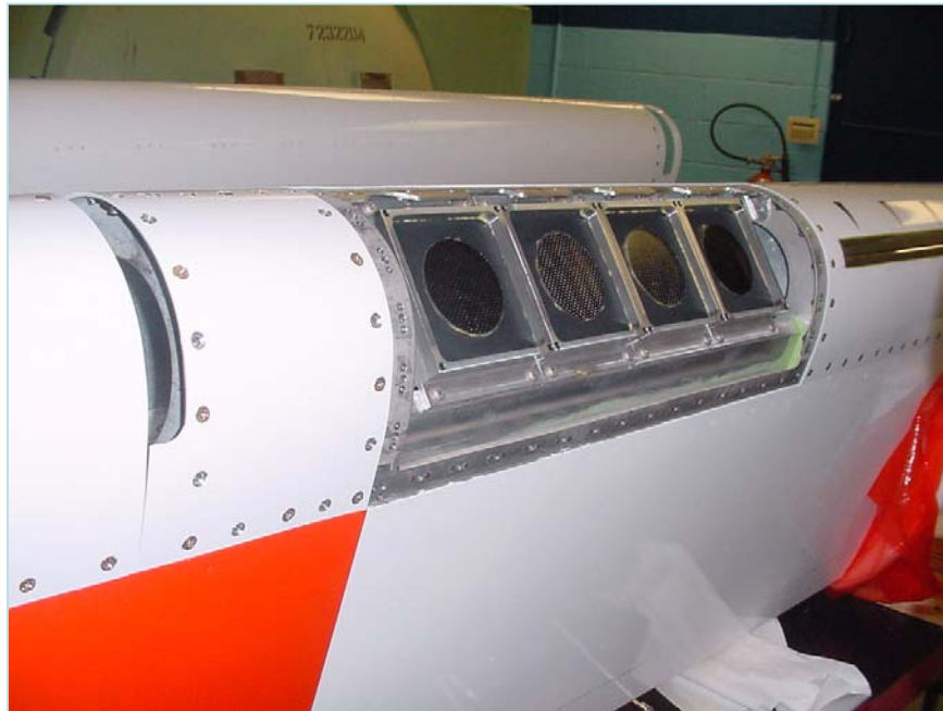
Figure 27: ATEAM-15 Actuators Installed in the XV-15 Flap.
