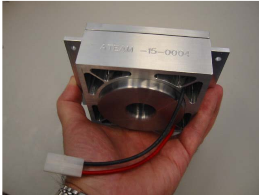
Figure 3: ATEAM-15 Actuator used for XV-15 Flight Tests.
